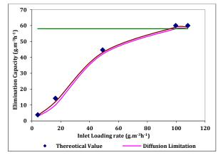
**Fig. 7** Comparison of ottengraf model and modified ottengraf model with experimental values for MEK removal in a Press mud based biofilter.
