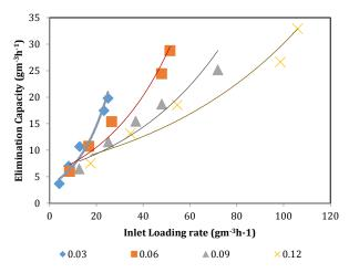
${\bf Fig.~6}$  Inlet Load Vs Elimination capacity for the removal of MEK  $\,$  using Press mud based biofilter  $\,$
