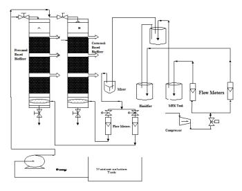
Fig. 1 Schematic diagram of biofilter
