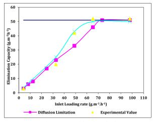
Fig. 8 Comparison of ottengraf model and modified ottengraf model with experimental values for MEK removal in a cornstack based biofilter.
