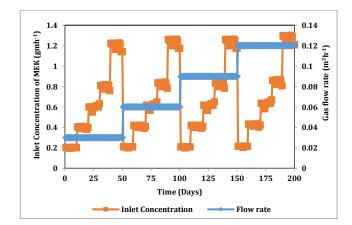
Fig. 2 Start-up of the biofilter for the removal of MEK using press mud based biofilter
