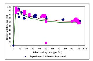
Fig. 9 Comparison of experimental and model predicted values for RE of MEK using Press mud and cornstack based biofilter.
