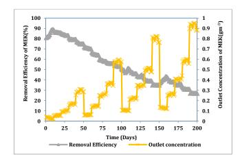
Fig. 4 Performance of biofilter for the removal of MEK using Press mud based biofilter
