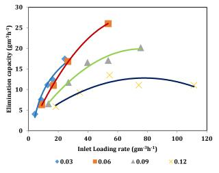
Fig. 5 Inlet Load Vs Elimination capacity for the removal of MEK  $% \mathcal{M}$  using press mud based biofilter
