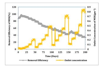
Fig. 3 Performance of biofilter for the removal of MEK using press mud based biofilter
